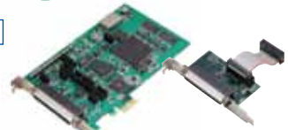
16ch Multiplexer Sub-Board ATCH-16A(PCI) Can add 16 single-ended or 8 differential inputs.
